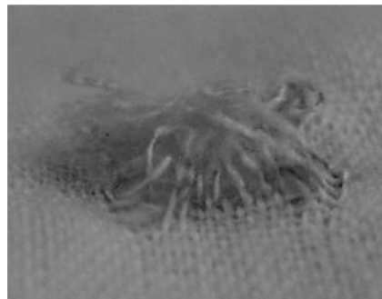
Fig. 13: Observed from the side of 92 pistol point domed bullet exit hole
