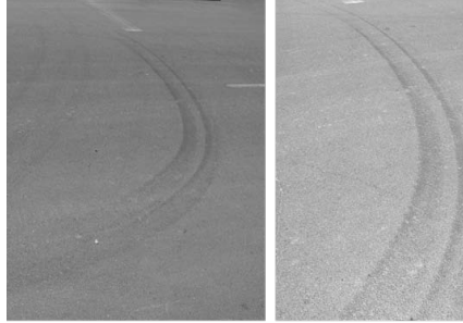
Figure 4 - The ABS-unequipped automobile tire sideslip trace
