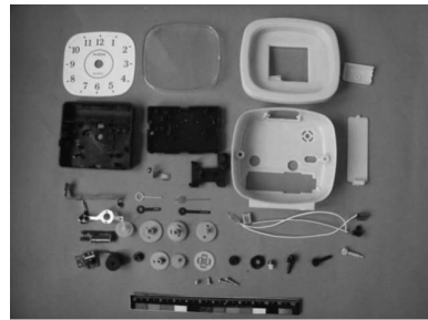
Figure4. Composition and morphology of quartz clocks
