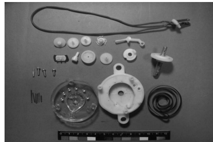
Figure 6 Composition and morphology of fan's timer
