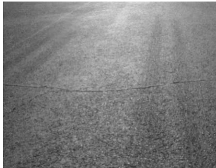
Figure 3 - The ABS-equipped automobile tire braking trace is light and discontinuous
